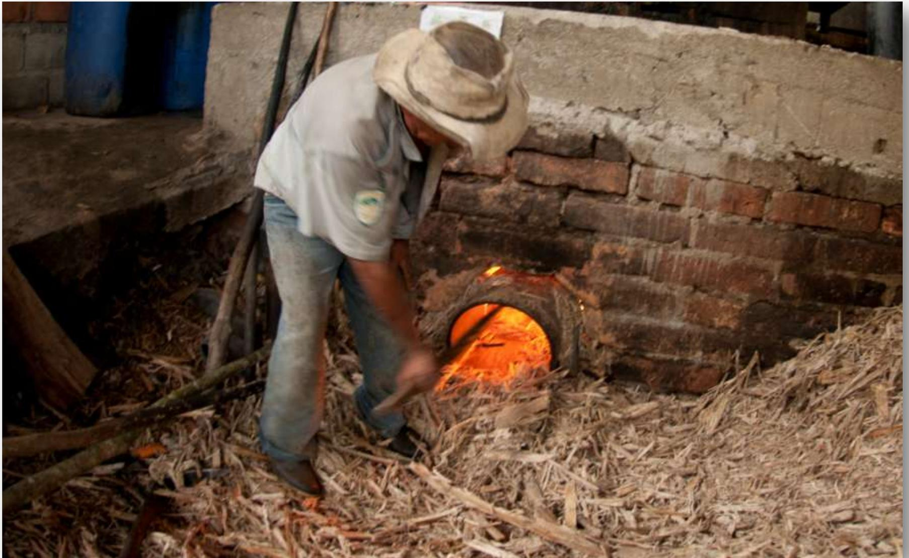
EL HORNO. COMBUSTIBLE BAGAZO Y CARBON MINERAL
